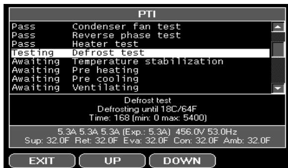
4. Press the **F2/F3** keys to scroll between each of the tests.
